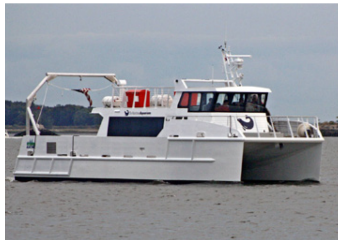
Maritime Aquarium at Norwalk's vessel 'Spirit of the Sound' equipped with BAE Systems HybriGen technology and Li-ion batteries for energy storage. Copyright: BAE Systems.
